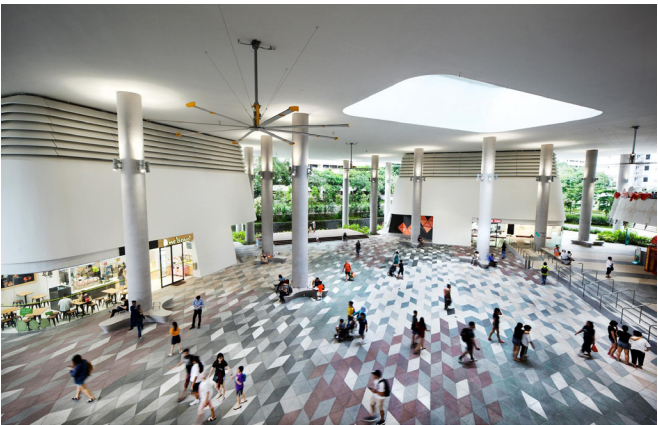
▲ Kampung Admiralty – The ground-floor Community Plaza incorporates passive design strategies, using shade, ceiling fans for ventilation, and daylighting from overhead openings. (Image credit: Patrick Bingham-Hall)
